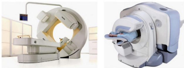
Fig. 1.4. Clinical SPECT/CT systems. (Courtesy: Philips and GE.)
